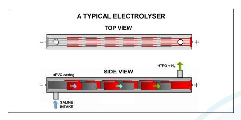
All anodes and cathodes are made of titanium. Anodes require a coating of mixed metal oxides (MMO) of the platinum group of metals. This coating is essential for the generation of chlorine and can last between 5 to 8 years (All our anodes are guaranteed for 5 years continuous duty)
